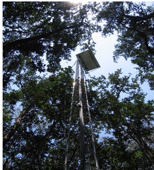
Figure 2-27. Photo of the canopy-scale eddy flux tower at the SRS-6 site (J.Fuentes & J.Zieman, UVA, PIs).
