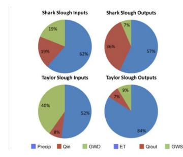
**Figure 5.6:** Pie charts of water budget components in Shark and Taylor Sloughs. Inputs include precipitation (blue), surface water inflow (red), and groundwater discharge (green). Outputs consist of evapotranspiration (blue), surface water outflow (red), and groundwater seepage (green). Values represent the average percentages of each component for Taylor Slough on a monthly basis between Jan. 2008 – July 2009, and on an annual basis in Shark Slough between 2002-2008.
