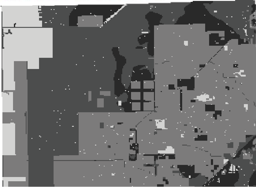
Figure 8.4: Sophisticated Redlands Excluded Layer used in SLEUTH calibrated urban growth simulation for Redlands. Lighter colors offer more resistance to development while darker colors offer less.
