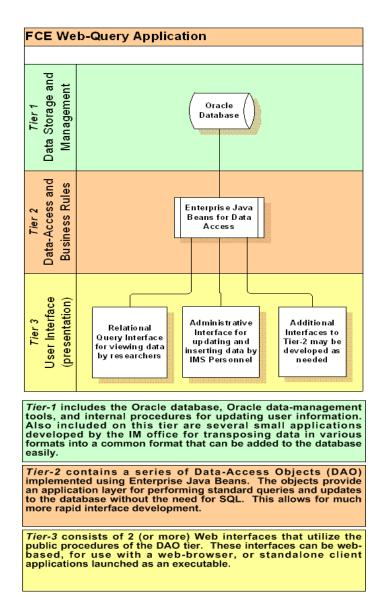
Figure III.D.1: Description of the 3-tiered web query application currently being developed and tested by FCE IM staff. This application will allow Oracle database access directly via the web with a fully interactive data query front end. It will also greatly facilitate database entry and updating procedures.
