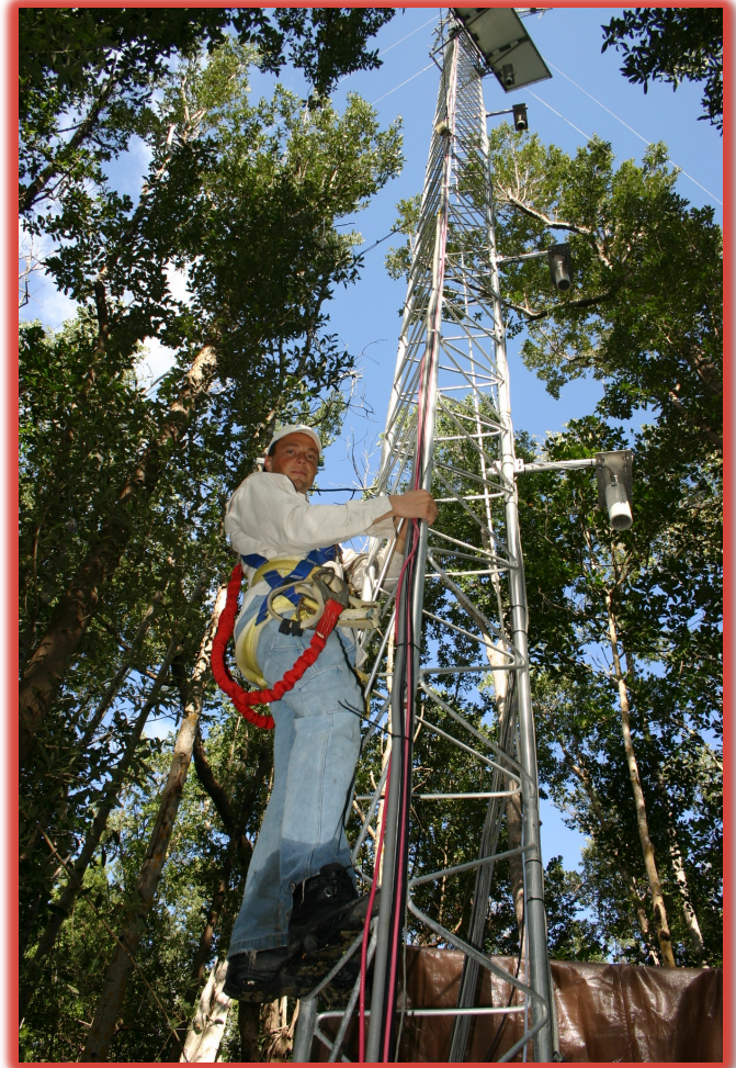
Figure 5:(above) Dr. Barr Scaling the Shark River Sough Eddy Covariance Flux Tower
