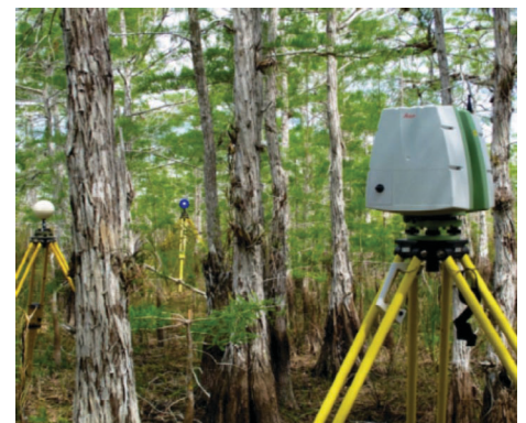
Above: Leica ScanStation C10 TLS and targets in Pine site.
